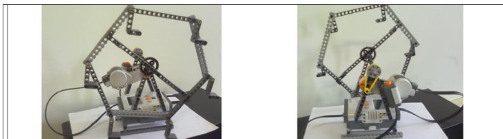
FIGURE 02 – Ferris wheel. View of the front (left) and back (right), where the sensor that starts movement can be seen.
