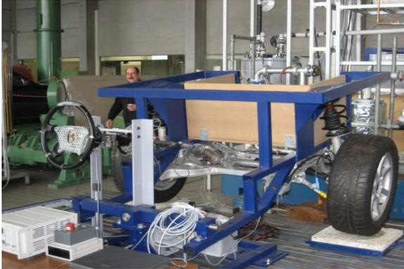
**Figure 7:** Test bench for steering system
