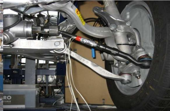
**Figure 8:** Steering track rod with strain gauges
